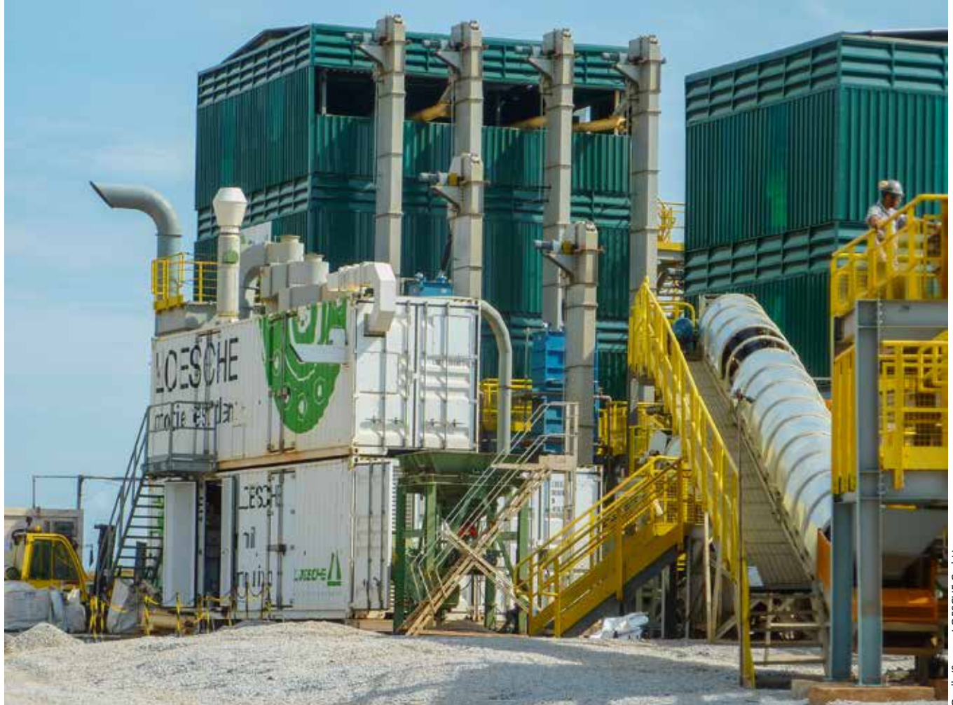
13 Loesche-Mahlanlage, in Containern transportabel • Loesche transportable containerised grinding plant
